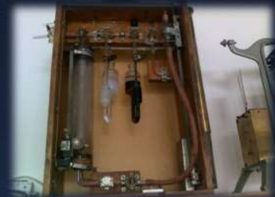
Scholander apparatus for measuring oxygen concentration in gas samples
