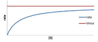
The Michalis constant and  $V_{max}$  parameters can be extracted in a number of ways. In the Lineweaver-Burk (Lineweaver & Burk, 1934) method, the reciprocal of the rate law is used to create a linear relationship.
