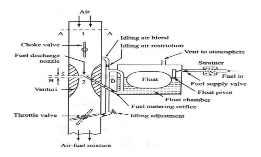
Applying the steady flow energy equation to sections AA and B–B  $_{a\eta q}$  assuming unit mass flow of air, we have,
