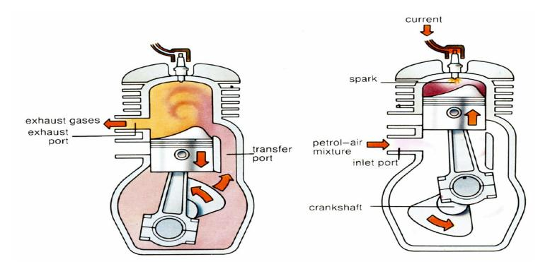
No piston stroke for suction and exhaust operations
