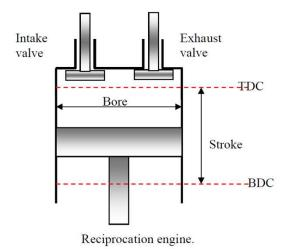
**Top dead center (TDC):** It is the dead center when the piston is farthest from the crank shaft. in HZ. Engine it is called inner dead center
