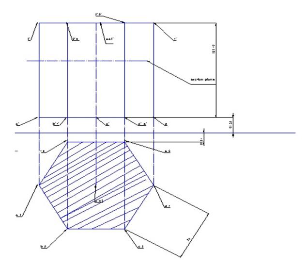
Q.2 A hexagonal base prism side 70 mm and height 119 mm ,axis perpendicular to HP cut by a section plane, section plane incline to HP at 35 degree and cut the axis 45 mm above the base. Sol.
