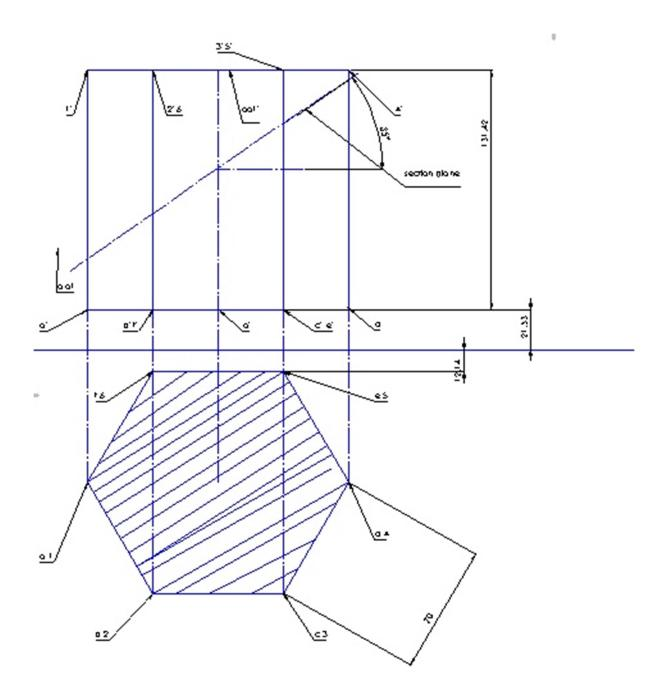
Q.3. A hexagonal base pyramided side 70 mm and height 119 mm ,axis perpendicular to HP cut by a section plane, section inclined to HP at 35 degree cut the axis 45 mm above the base.
