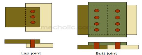
2. Butt joints (the plates are brought to each other without forming any overlap. Riveted joints are formed between each of the plates and one or two cover plates).
