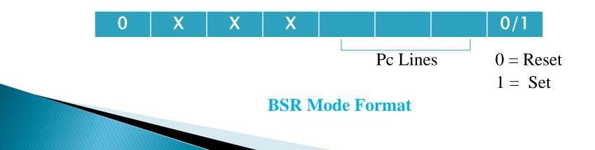
Example – To send Logic 1 on Pc<sub>2</sub> line.
