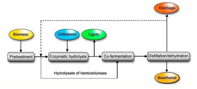
Separate hydrolysis and co-fermentation (SHCF)
