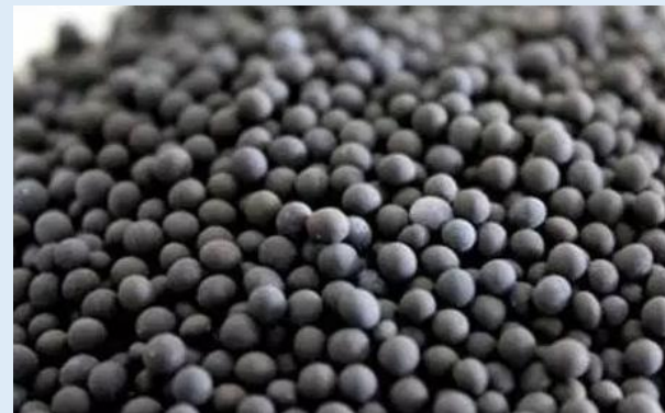
Pt on \text{Al}_2\text{O}_3 spherical pellets
