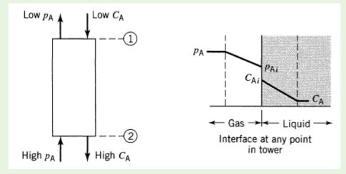
$F_l = \frac{F_l' C_U}{C_T}$  = downward molar flow rate of inerts in the liquid (mol/s)
