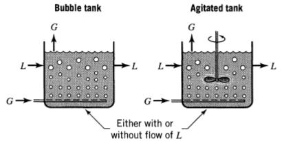
(b) Tanks – Bubble tank, Agitated tank
