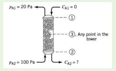
The value of  $C_{A_2}$  can be calculated from  $C_{A_2} = 0.08 p_{A_2} - 1.6 = 0.08 \times 100 - 1.6 = 6.4 \text{ mol/m}^3$ The tower height is then determined in the following way,
