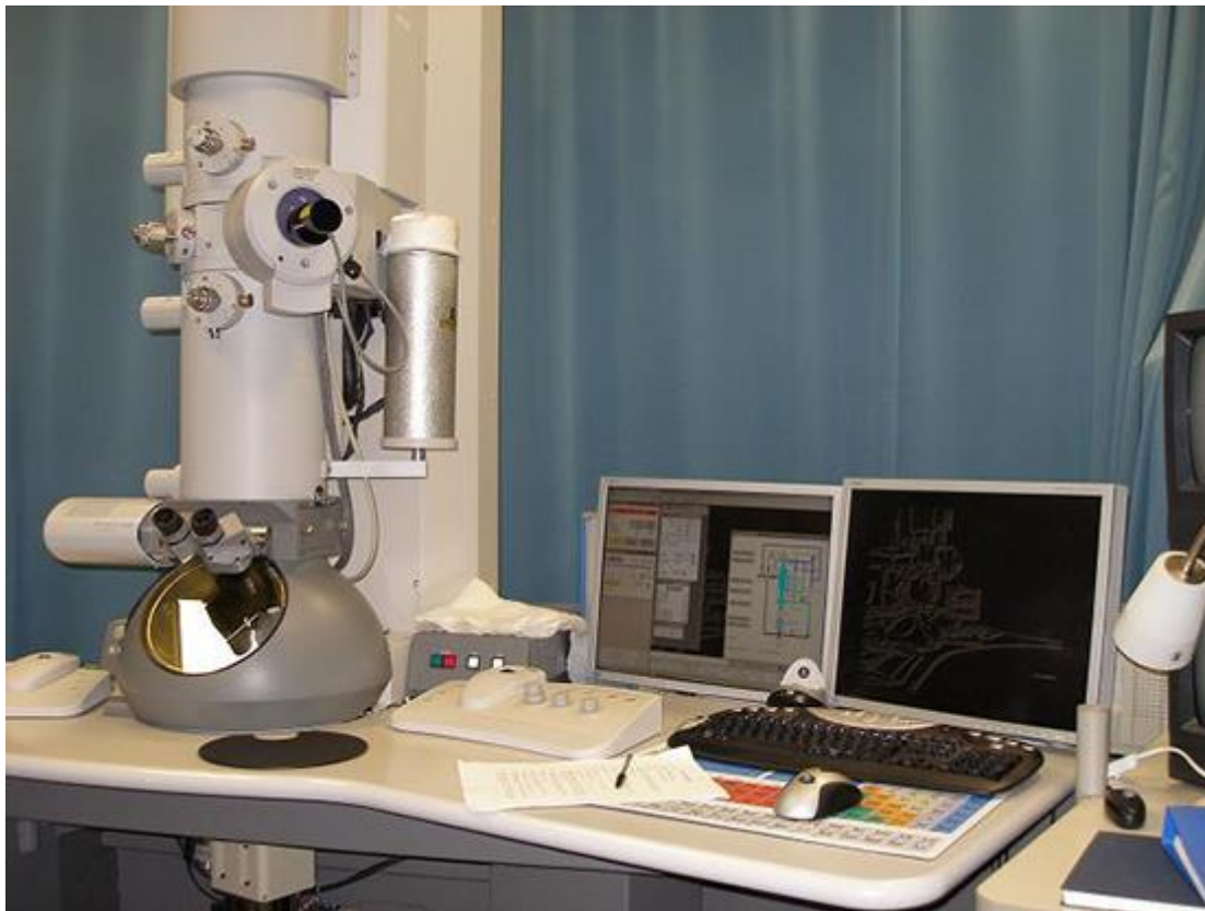
Figure 2.21 A transmission electron microscope (TEM).
