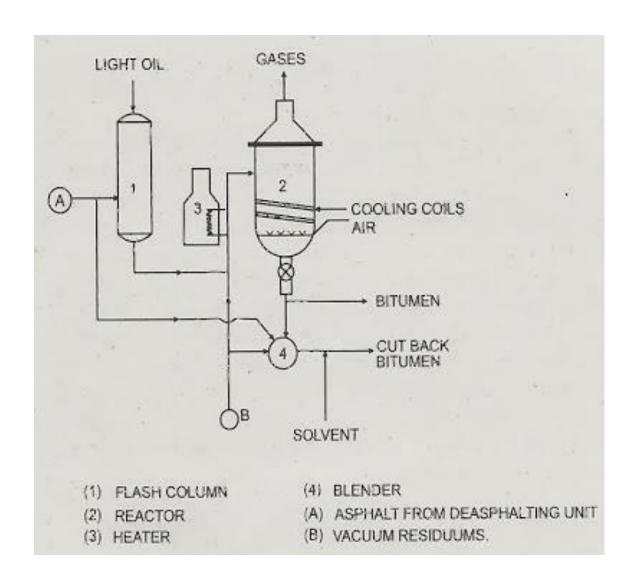
Batch process for bitumen manufacture
