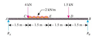
**Solution.** Given: Span (l) = 6m
