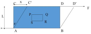
Shear strain is the distortion produced by shear stress on an element or rectangular block as above. The shear strain,  $\gamma$  (gamma) is given as:
