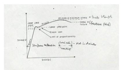
Fig: Behaviour of mild-steel rod under tension.
