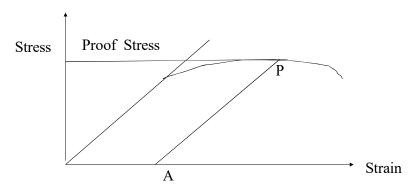
The proof stress is obtained by drawing AP parallel to the initial slope of the stress/strain graph, the distance, OA being the strain corresponding to the required non-proportional extension e.g. for 0.05% proof stress, the strain is 0.0005.
