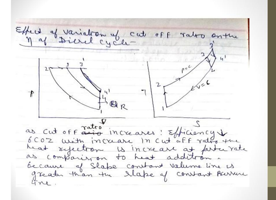
Comparison of otto cycle and sierel cycle. care >1 Same & comprision ratio and heat 10= EXtry 43010 head rejection 1-2-3'4' - Divel DieSelcycle
