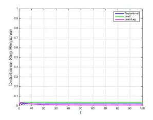
Lead-lag has better performance than lead due to larger low-frequency open-loop gain
