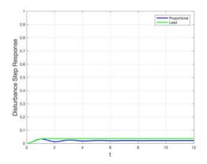
Disturbance response of lead design is worse due to smaller low-freq. open loop gain
