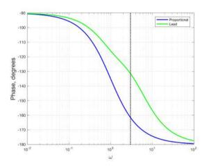
Observe additional phase from lead compensator and improved phase margin
