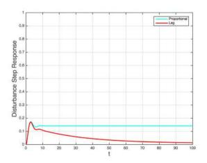
Larger low-frequency open-loop gain of lag design yields better step disturbance rejection
