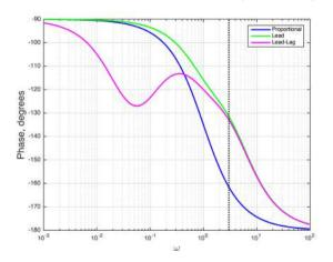
Observe additional phase from lead compensator and improved phase margin. By design, lead-lag does not reduce this much.
