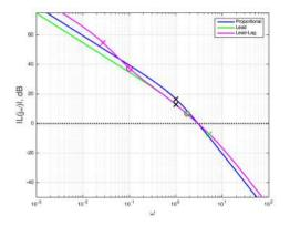
Black x: frequency of plant pole; Green x and circle: frequencies of lead compensator pole and zero Magenta x's and circles: freq's of lead-lag compensator poles and zeros Same cross over frequency; lead and lead-lag have shallower slope Lead-lag has larger low-frequency open-loop gain
