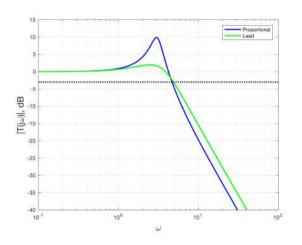
Note reduction in resonant peak (reflects larger damping ratio)
