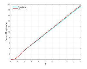
Lag has reduced steady-state error, by design
