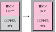
Two bodies reaching thermal equilibrium after being brought into contact in an isolated enclosure.
