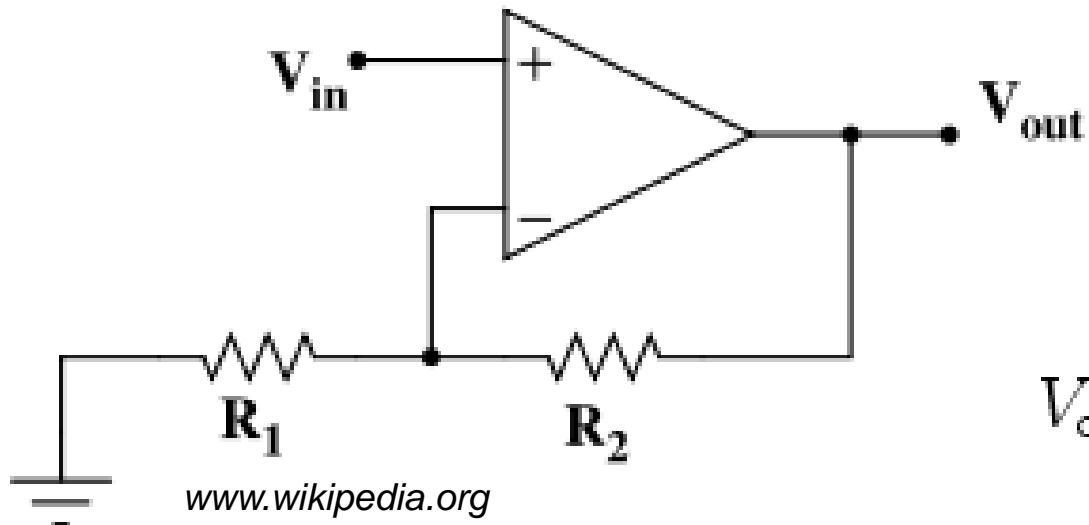
$$V_{out} = V_{in} \left( 1 + \frac{R_2}{R_1} \right)$$
