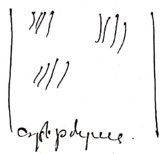
Cryst. polymer embedded in an amorphous matrix.
