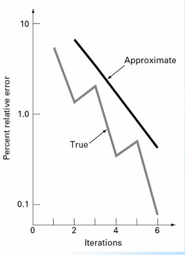
Benefit of the bisection method is that the number of iterations required to attain an absolute error can be computed a priori—i. e., before starting the iterations.
