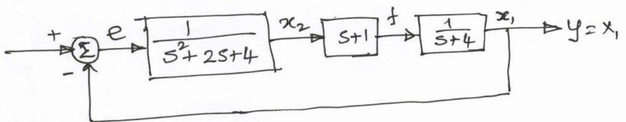
Note that the output of  $(S+1)$  is given a dummy variable, while output of  $1/s$  or  $1/s^2$  terms is assigned a state variable.
