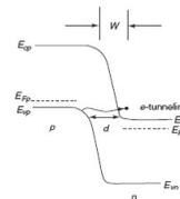
Reverse bias with electron tunnelling from p to n leads to Zener breakdown
