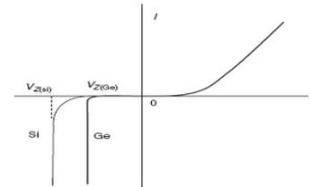
Comparison of Zener breakdown of Ge and Si semiconductor diodes with respect to I-V curve
