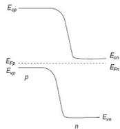
Energy band diagram of a Zener diode
