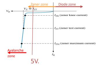
This curve illustrates the minimum and maximum ranges of current operation that the Zener can effectively maintain its voltage.
