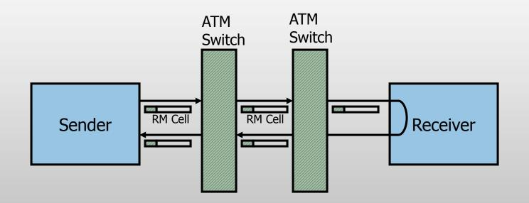
• SENDER TRANSMITS CELLS AT THE ACR (ACTUAL CELL RATE) WHERE MCR <= ACR <= PCR
