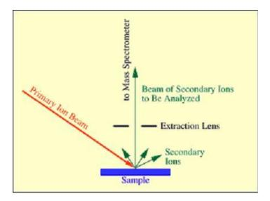
These ions are then accelerated, focused, and analyzed by a mass spectrometer.
