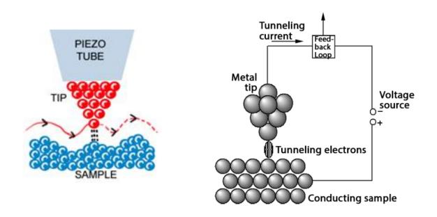
Feedback loop and electron tunneling for scanning tunneling microscopy (STM)
