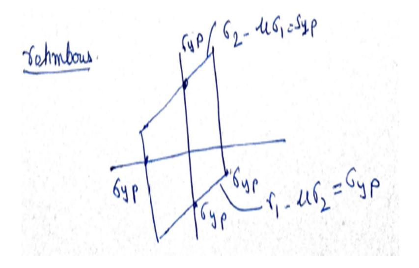
Mag Storin Enorgy theory A Failure or yieding occurrat point in a member when the Strain Energy/unit member Volume Ing bigorial Stress system reaches. the limiting Strain Energy ploranit valume as determined from Simple Tonion Wet.
