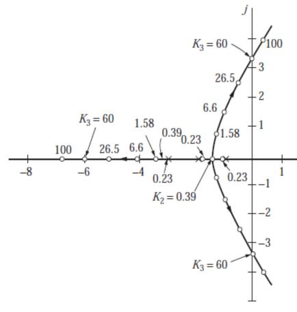
Notice that there are three loci or *branches* corresponding to the three roots and that they "emerge" or begin (for K=0) at the poles of the open-loop transfer function (-1, -2, -3).
