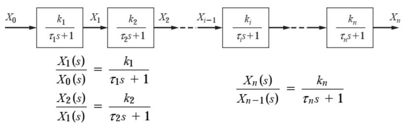
Overall transfer function, we simply multiply the individual transfer functions;
