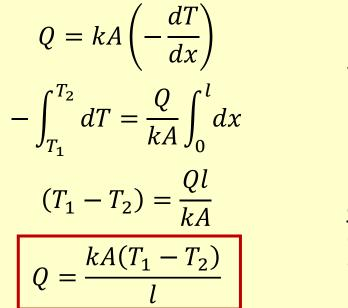
where k = thermal conductivity, (W/mK)  $\frac{dT}{dx}$  = temperature gradient  $\frac{dT}{dx}$  is negative as temp at x = 0 > temp at x = l
