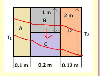
Thermal resistances of slab B ( $R_B$ ) and C ( $R_C$ ) are parallel and they together is in series with the resistances of A ( $R_A$ ) and D ( $R_D$ )
