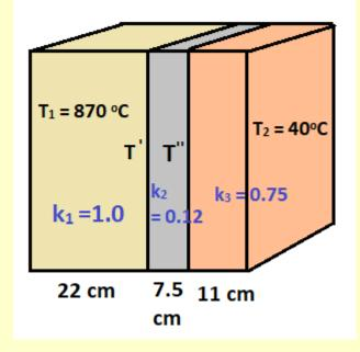
(b) As the rate of heat conduction through each layer is equal
