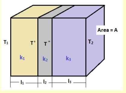
$$Q = \frac{\Delta T}{(R_1 + R_2 + R_3)}$$
