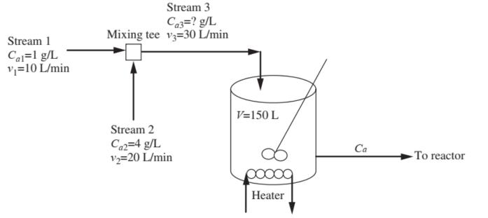
We can model the mixing tee and the blending tank using an unsteady-state mass
