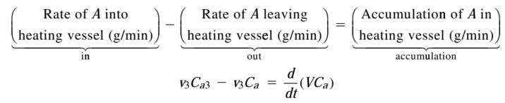
Volumetric flow rate v is constant into and out of the heating vessel at  $v_3$ . Thus the volume of fluid in the tank V is constant.
