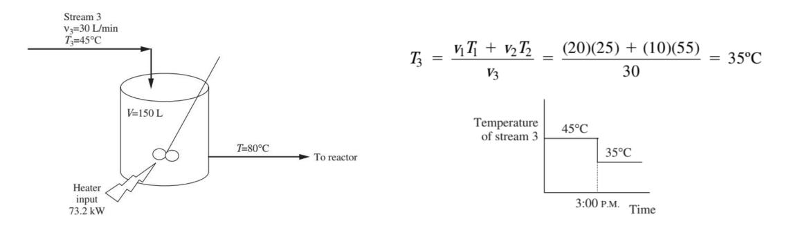
To determine the effect of this inlet temperature disturbance on the feed to the reactor, an unsteady-state energy balance on the heating vessel is required.
