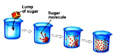
Diffusional mass transfer occurs in the absence of any macroscopic motion of the medium through which such transfer takes place. As a result, diffusional mass transfer is a very slow process.
