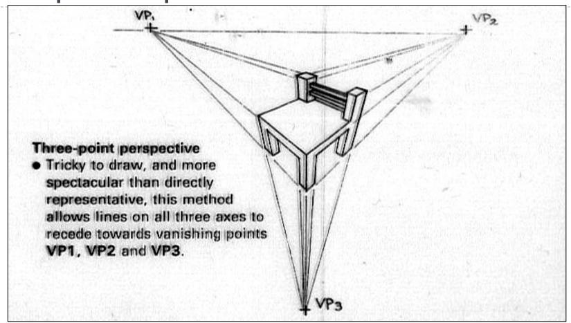
No system of parallel edges with picture plane, three VP
