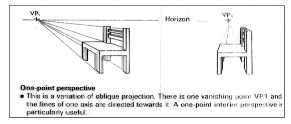
One face of object is parallel to picture plane, one VP
