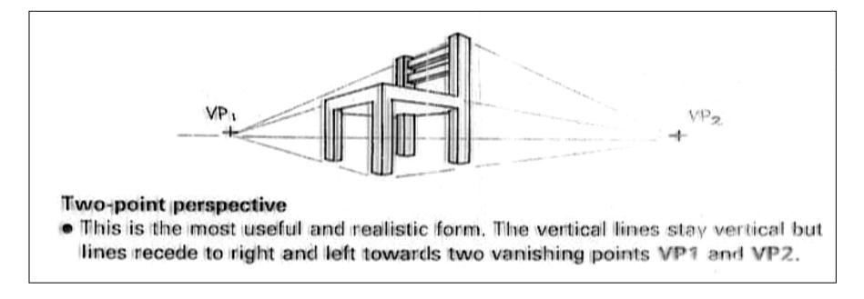
Object at angle with picture plane, but vertical edges are parallel to picture plane, two VP
