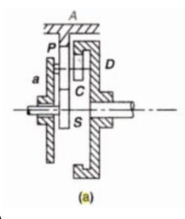
Gear P, Gear – A, arm constitute internal epicyclic gear train.
