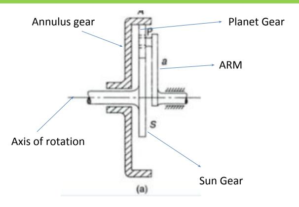
Sun Gear: Sun gear rotates about fixed axis of rotation.
