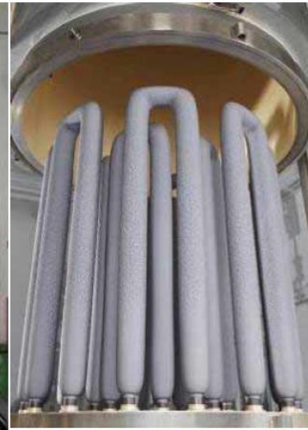
As grown polysilicon rods after a reactor run
