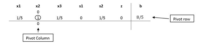
III. In order to keep the tableau equivalent, the other variables not contained in the pivot column or pivot row must be calculated by using the new pivot values. For each new value, multiply the negative of the value in the old pivot column by the value in the new pivot row that corresponds to the value being calculated. Then add this to the old value from the old tableau to produce the new value for the new tableau. This step can be condensed into the equation on the next page:
