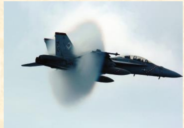
Vapor cloud around an F/A-18F Super Hornet as it flies near the speed of sound.
