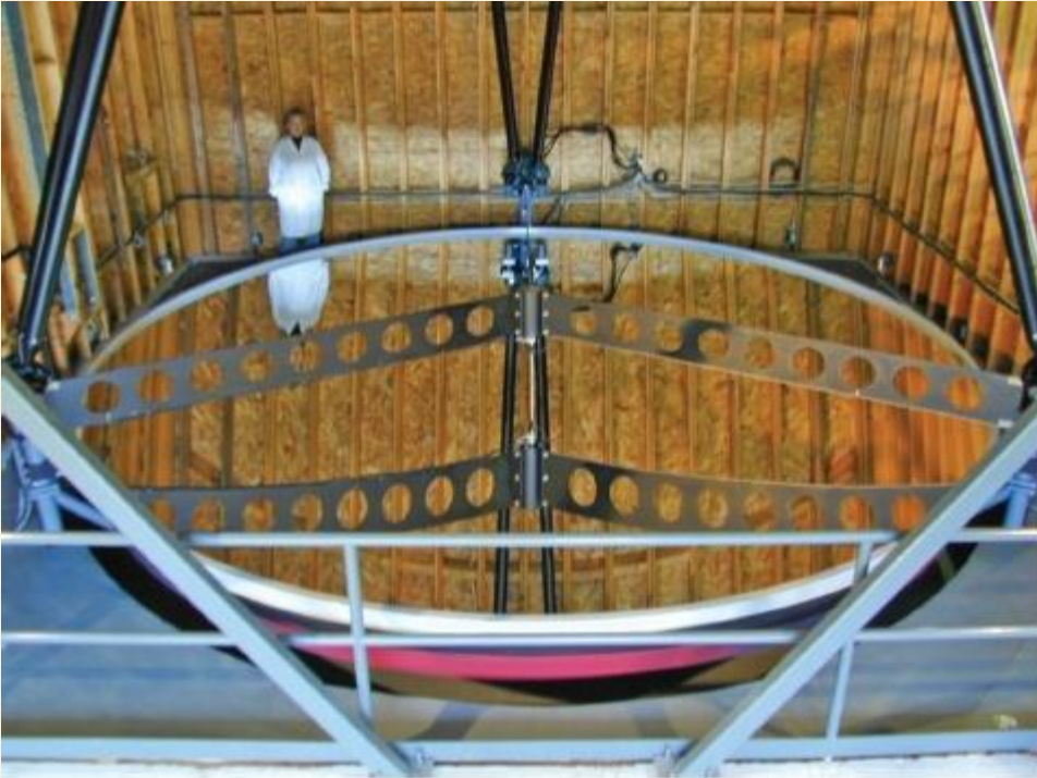
The 6-meter spinning liquid-mercury mirror of the Large Zenith Telescope located near Vancouver, British Columbia.
