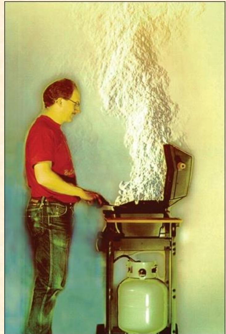
Schlieren image of natural convection due to a barbeque grill.
