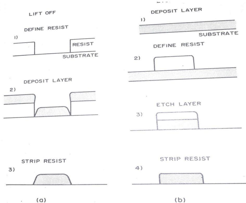
A schematic representation of two techniques for transferring resist features into a layer. (a) Shows the resist/deposition strip sequence of lift off, and (b) shows the deposit/resist/etch/strip sequence of etching.
