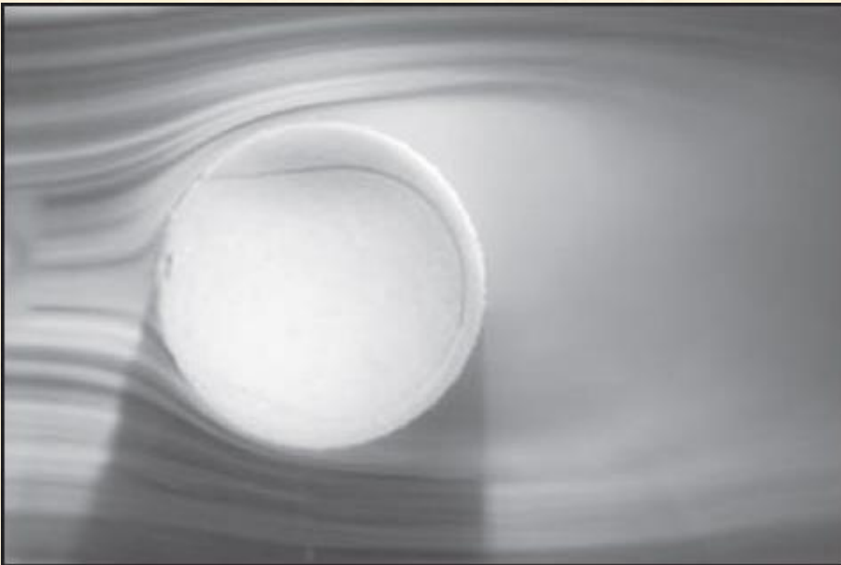
External flow over a tennis ball, and the turbulent wake region behind.
