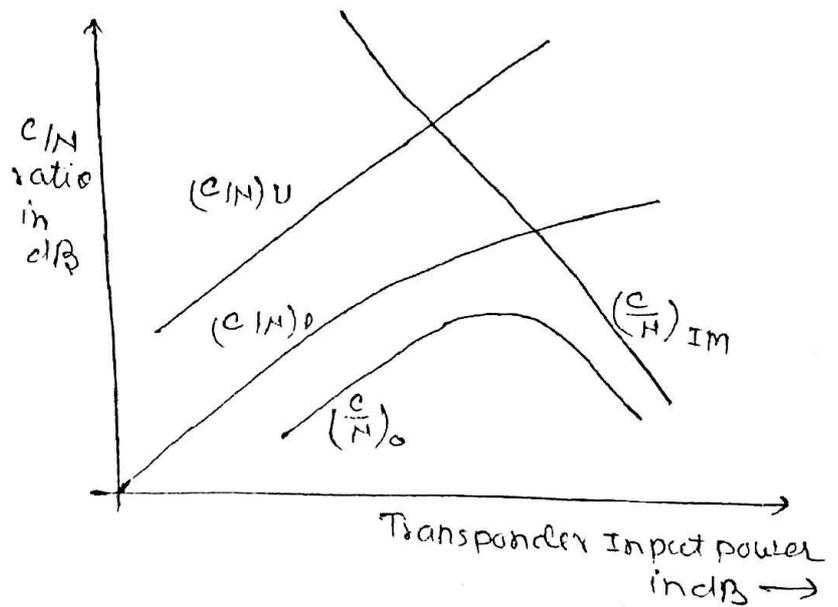
$\rightarrow$   $\frac{C}{N}$  ratio for a link using nonlinear Transponder  $\leftarrow$
