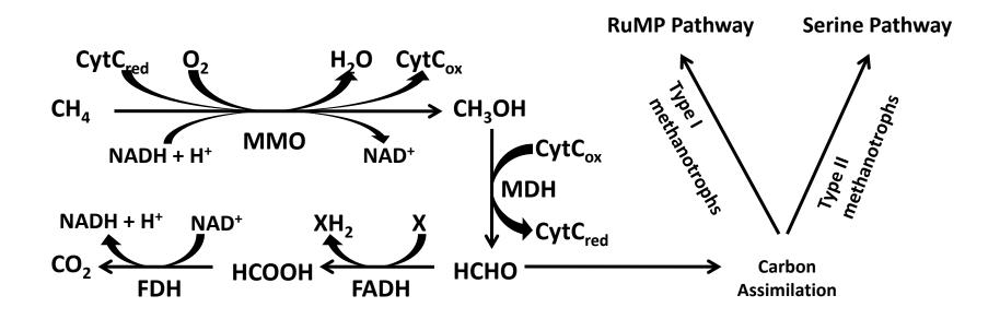
Where, MMO: Methane monooxygenase; MDH: Methanol dehydrogenase; FADH: Formaldehyde dehydrogenase; FDH: Formate dehydrogenase; RuMP: Ribulose monophosphate; NADH: Nicotinamide adenine dinucleotide; CytC: Cytochrome c
