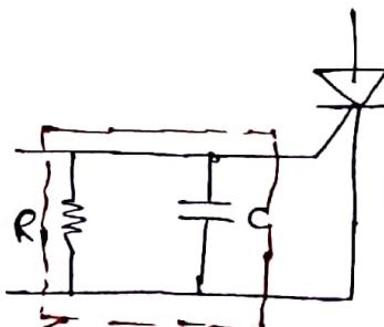
RC circuit to filter out noise.
