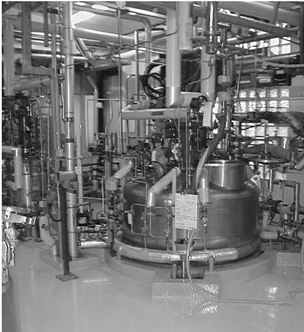
Photograph of production fermentation facility used for expressing recombinant protein in an E. coli expression system
