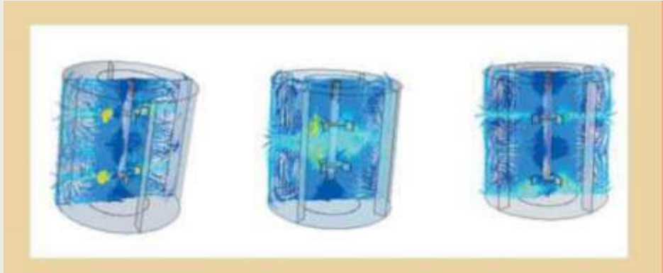
(a) stirred tank, radially pumping impellers; (b) stirred tank, closely placed impellers; (c) stirred tank, impellers too far apart.
