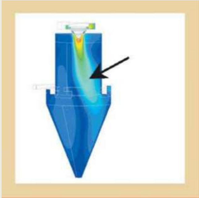
Spray dryer, velocity field
