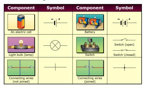
Symbols are used to represent the various electrical components in circuits.
