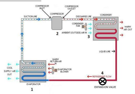
To avoid continuous running of electric motor (motor required to run the compressor) and unnecessary work of compression, thermostatic control is used which senses the set interior temperature and stops the motor from running and when the temperature rises again, the motor restarts and the Compressor starts working again.
