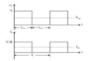
$V_{dc} = A \text{verage value of output or load voltage.}$   $I_{dc} = A \text{verage value of output or load current.}$   $t_{ON} = \text{Time interval for which SCR conducts.}$   $t_{OFF} = \text{Time interval for which SCR is OFF.}$   $T = t_{ON} + t_{OFF} = \text{Period of switching or chopping period.}$  $f = \frac{1}{T} = \text{Freq. of chopper switching or chopping freq.}$
