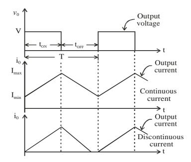
Expressions for Load Current *Io* for Continuous Current Operation When Chopper is ON ( $0 \le T \le Ton$ )
